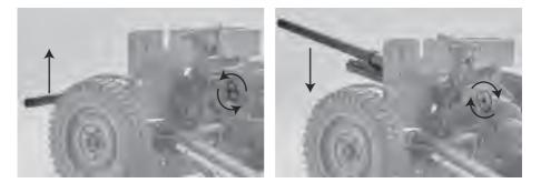
Adjust the Left/Right firing direction of the gun by rotating the indicated control clockwise or 7. anti-clockwise as shown in the diagram 使用涡轮蜗杆减速的方向机调整方向射界;
